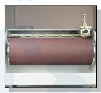
Pack sandpaper outside the surface of roller. The sample is pressed against the roller with sandpaper, which makes sample lateral moving along roller.
